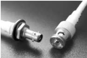
Figure 3. Bayonet triaxial connectors
